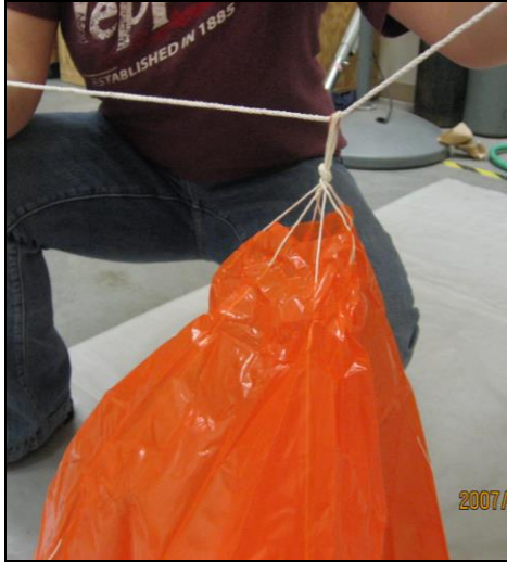
Figure 14 - Pull cord through four loops at the top of the parachute
