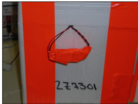
Figure 26 -Once connected wrap cables with tape
