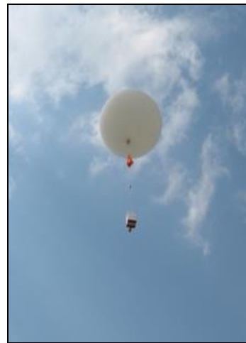
Figure 32 - Release the ozonesonde
