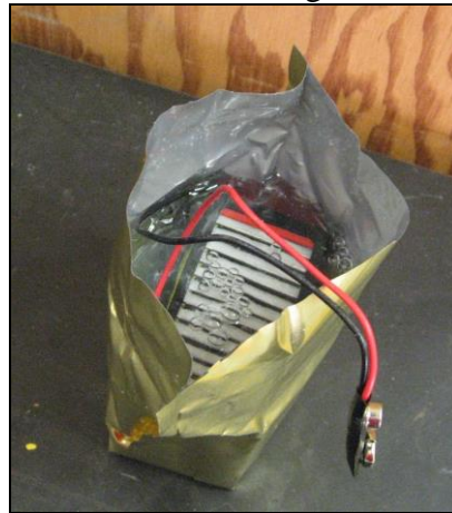
Figure 23 - Wet battery bag with water filled above the battery
